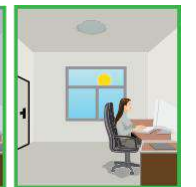
Light will switch off automatically even with presence detected, if the nature light is sufficient.
