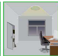
People left, light dims to 0/10%/30%/50% (options) standby level after the hold time.
