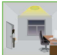
With insufficient natural light, the sensor switches on the light automatically when person enters room.
